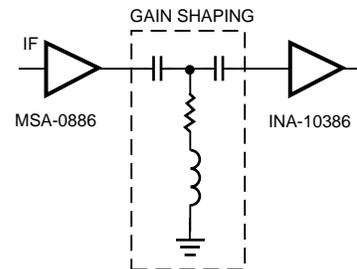
**Figure 9. IF Amplifiers using INA MMICs**
