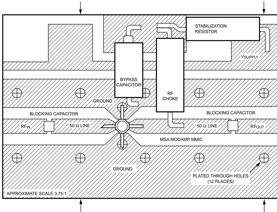
**Figure 6. Typical MODAMP MMIC Circuit (dual ground configuration)**
