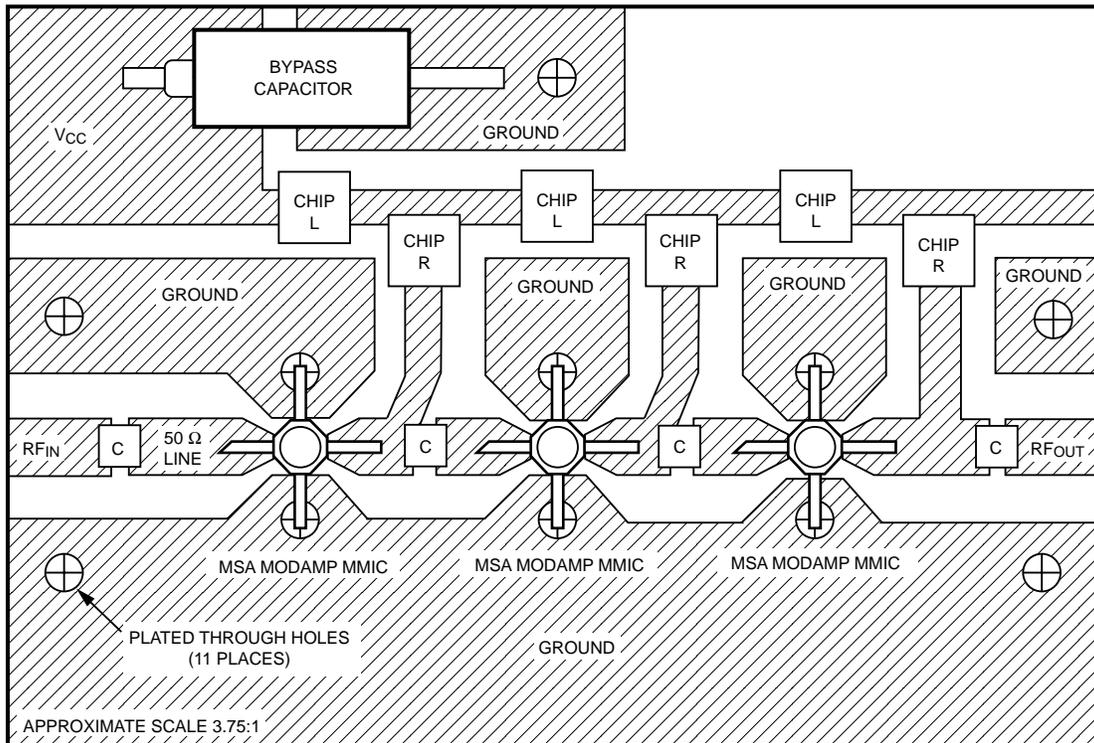
Figure 7. MODAMP MMIC Circuit Layout (three stage cascade)
